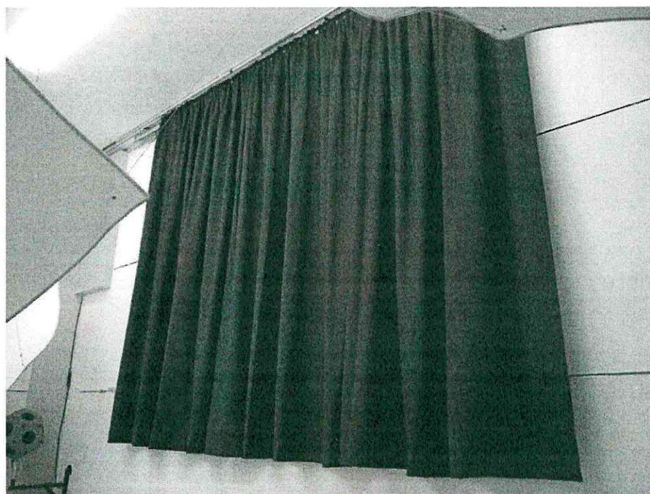
Figure B.2. Test arrangement in the reverberation room (oblique view).
